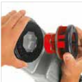
Easy insertion of the die heads
