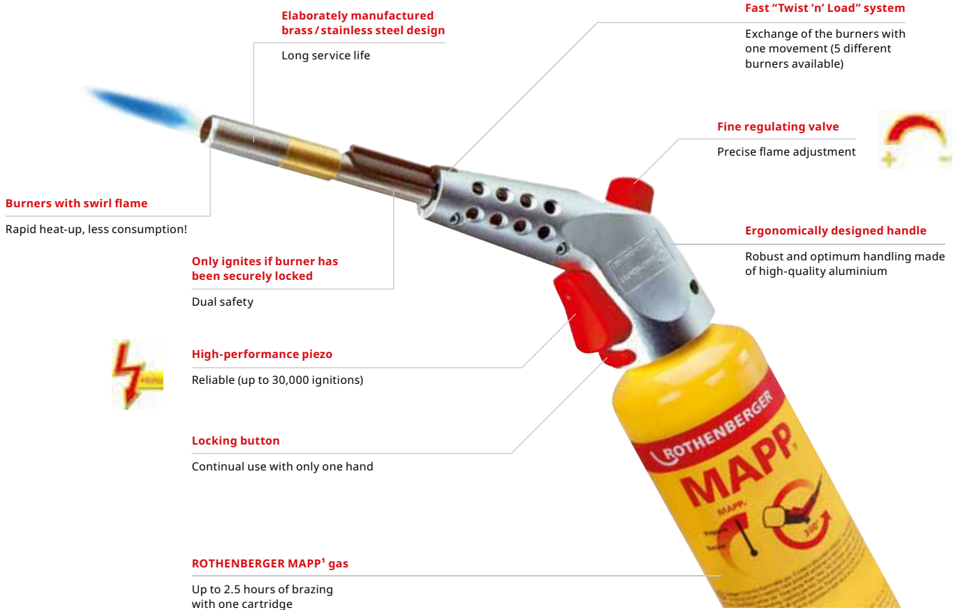
High flame temperature based on cyclone swirl
