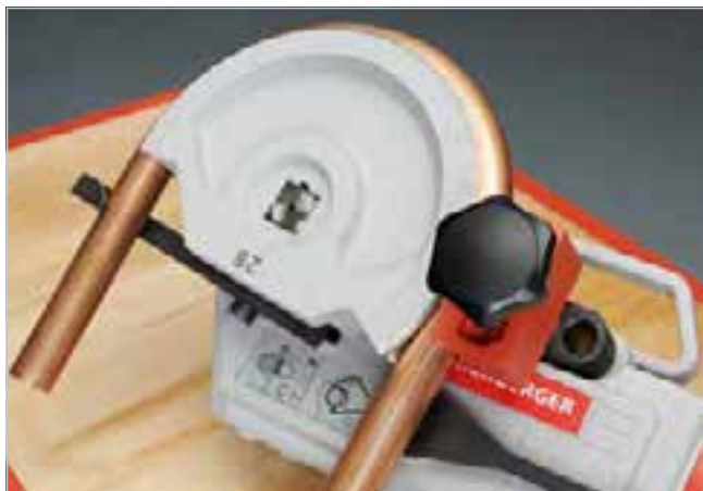
Forged aluminium segments with bending angle scale
