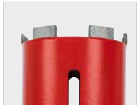
Air vents for removal of the drill dust and for cooling work
