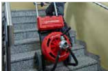
Easy transport due to stair capable chassis
