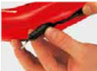
Removable internal pipe deburrer
