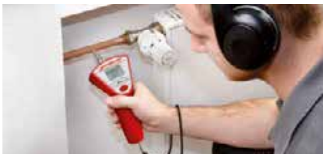
Acoustic leak detection of heating installations
