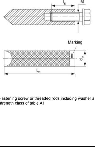
Marking: anchor size e.g.: M10 Stainless steel in addition A4 e.g.: M10 A4 High corrosion-resistant steel in addition C e.g.: M10 C
